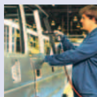
Bohrmaschine 260 l/min, 6-7 bar
